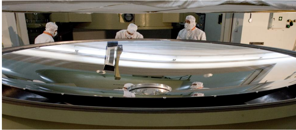
Figure 5.3 Herschel's 3.5m mirror being coated
