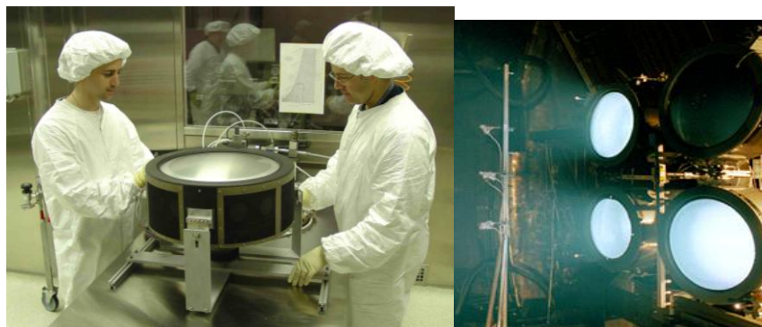
Figure 6.1: The NEXT Thruster and Multi-thruster testing.
