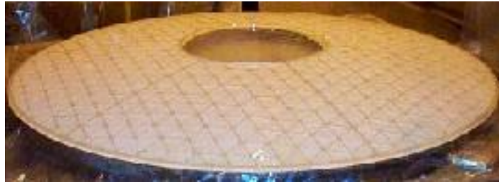
Figure 5.1: ITT's 2 meter class Mirror Demonstrator
