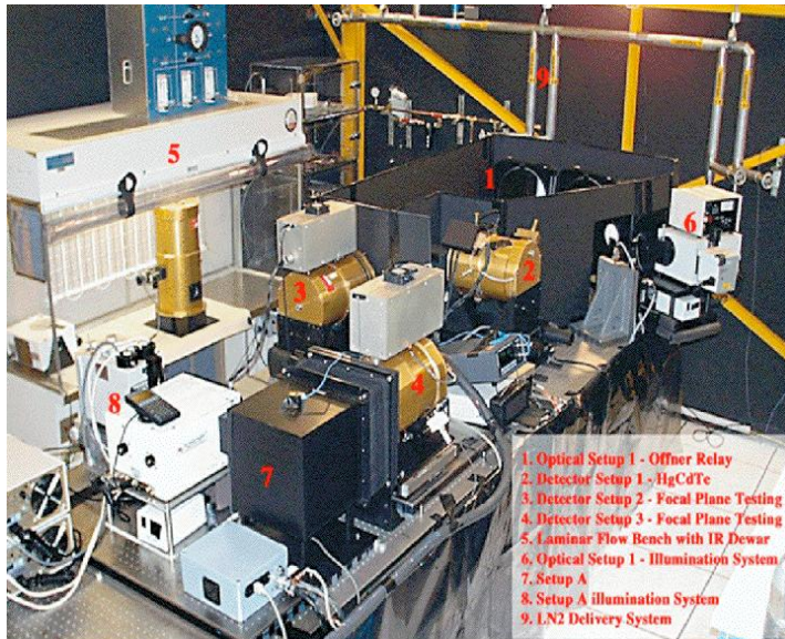
Figure M-6: GSFCL DCL WFC3 test setup.
