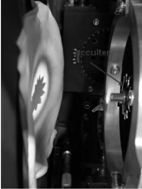
Figure 7: On the right is the test starshade mounted in a ring by guitar strings. On the left a cloth has been placed in the system so that the light distribution and the shadow of the starshade can be seen.
