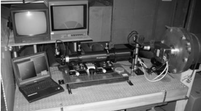
Figure 9: The setup on the detector end is shown. The science detector is mounted up against the end of the vacuum tube on the right. There is a small telescope, another small camera, two monitors for use in aligning the system. The laptop on the left will be used to take the data.
