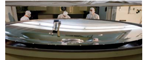
Calor Alto 4-m coating chamber with 3.5-m Herschel PM
