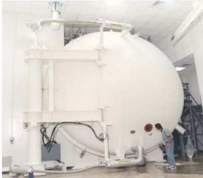
SOMTC 5.5-m (4.57-m clear zone) coating chamber
